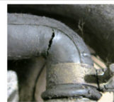
M110/M116/M117 Position of engine airduct rubber components underneath suction manifolds
